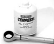
The Tempest AA472 oil filter torque wrench is a great addition to any toolbox. Its 1" hex allows easy installation or removal of all oil filters. The torque wrench also comes present to 17 foot pounds and is easily recalibrated. P/N 08-07023 .....
